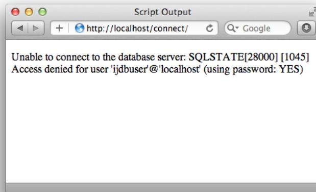
Figure 4.8. The detailed error message resulting from an incorrect password
